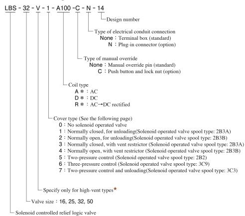
★Use high-vent pressure types if the shifting time from unloading to on-loading is reduced.
